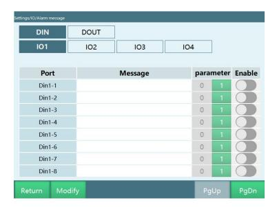
For example: set the IO emergency stop signal port to 15 to connect to the anti-collision IO, 1 to trigger and 0 to release; if DIN1 is triggered, it will report "Robot 1 IO emergency stop is triggered"; at this time, find DIN1 on the alarm message interface, and enter "Trigger anti-collision" in the message field, then triggering DIN15 again will report an error "Trigger anti-collision" instead of "Robot 1 IO emergency stop is triggered".
