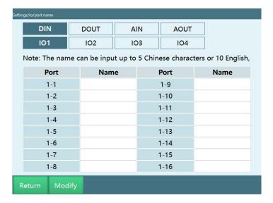
If the name of DIN1-1 is set as "enable ", the DIN1 name "enable " will be displayed in the [IO] of [Status]
