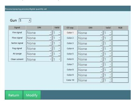
After clicking "Modify", the "Modify" button changes to "Save", and the selection box turns white. At this time, you can select the gun number, and select the port, effective value and color number after the respective functions. Please use the 16-bit RGB format for the color number. After filling in the color number, the corresponding "Color oil circuit" box will change to the corresponding color.
