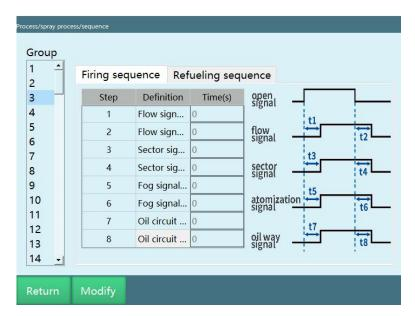
This is the refueling sequence, and the time to be set for each signal on the left corresponds to the sequence diagram on the right. The air purge, clean solvent, and fire signals correspond to the ports set in the digital setting. (As shown below)
