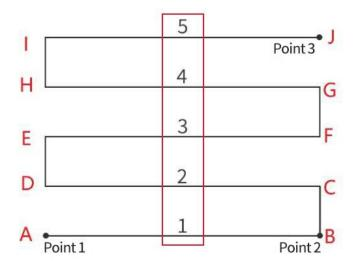
Set the number of layers to 2, additional times to 1, then the spray gun will operate in the sequence of points  $A \rightarrow B \rightarrow A \rightarrow D \rightarrow C \rightarrow D$ ;
