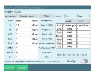
At present, the polishing process only supports polishing in the straight line direction. Compared with the MOVL instruction, the POLISH\_EDGE in the polishing process adds
