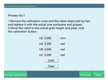
Step 2: Remove the calibration cone and the robot pointed tool hand and replace it with the actual workpiece and gripper; run the robot to the actual grasping height and attitude, and click the [Calibrate] button.
