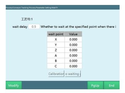
Waiting delay: determine whether there is a workpiece within 0.5s, and continue to track if there is a workpiece. If there is no workpiece, the robot will go to the waiting point
