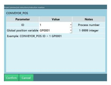
When this instruction is executed, the sensor calibration result of the conveyor belt process number 1 is stored in the global point GP001.
