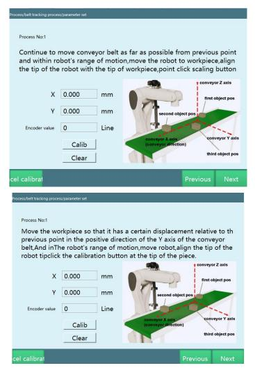
Step 1: Place a pointed calibration cone on the conveyor belt, move the conveyor belt so that the calibration cone on the conveyor belt moves within the motion range of the robot, move the robot to the workpiece so that the robot tool end tip is aligned with the tip of the calibration cone, click [Calibrate].
