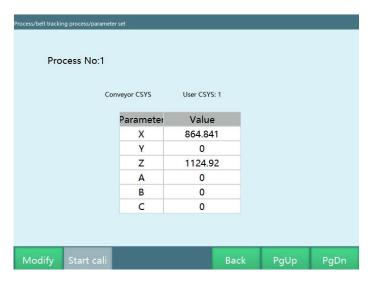
Conveyor belt coordinate system calibration: calibrate 3 points, calculate the user coordinate system of the conveyor belt; click [Modify], and then click [Start calibration] button to enter the calibration interface
