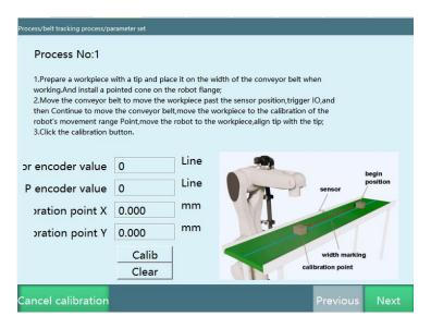
Step 1: Prepare a workpiece with a tip, place it at the width of the conveyor belt at work, and install a pointed cone on the robot flange; move the conveyor belt so that the workpiece moves past the sensor position, trigger IO, then continue to move the conveyor belt to move the workpiece to the calibration point within the robot's range of motion, stop the conveyor belt, move the robot to the workpiece so that the tip aligns with the tip; click the [Calibrate] button.
