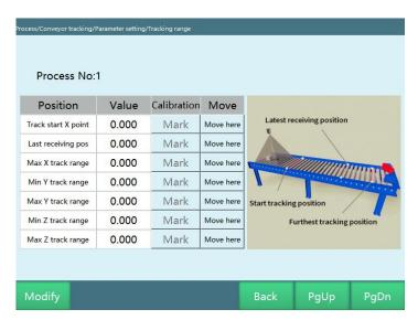
This interface is used to set some key positions and tracking range of the robot during the tracking process
